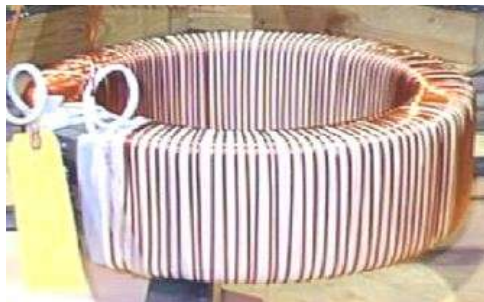
Figure 2 (b) Equivalent magnetic circuit Figure 3: Photograph of “cut” CT core with distributed winding around the core
