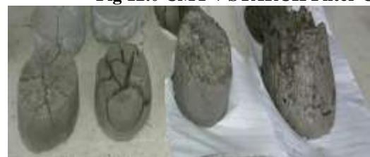
Fig 14.0 CMT + XC-POLYMER Filter Cake
