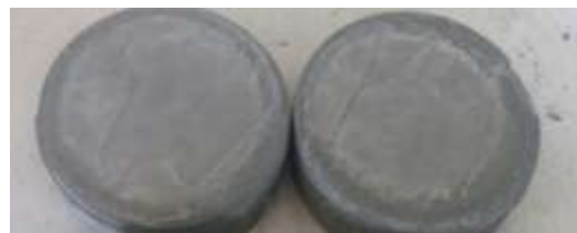
Fig 12.0 CMT + STARCH Filter Cake
