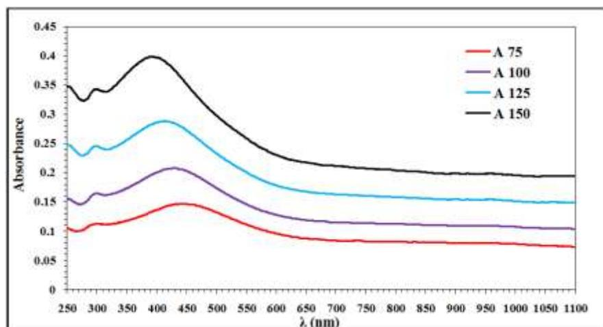
**Fig. 5:** Absorbance spectrum for colloidal Ag-Au Nano particles produced by exploding wire with different current.
