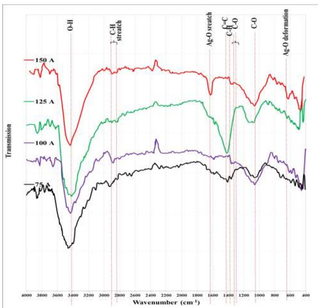
**Fig. 6:** FTIR patterns for Ag-Au Nano particles produced by exploding wire with different current.
