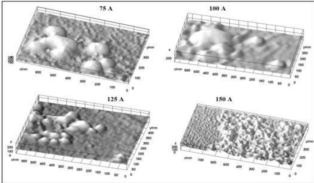
**Fig.3:** SEM images for the produced Ag-Au Nano particles by exploding wire with different current
