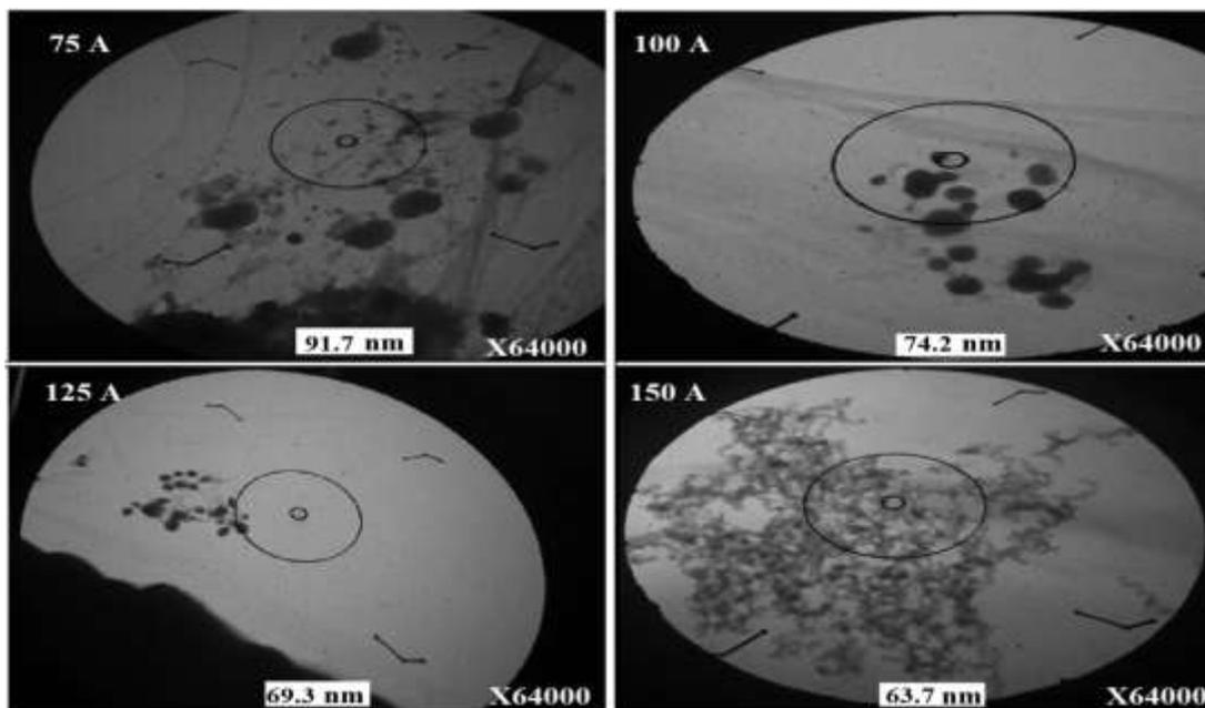
**Fig.4:** TEM images for the produced Ag-Au Nano particles by exploding wire with different current
