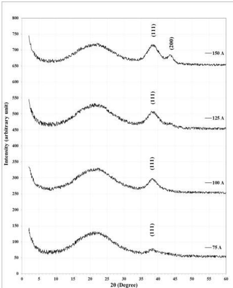
Fig.2: XRD patterns for producing Ag-Au Nano particles by exploding wire with different current
