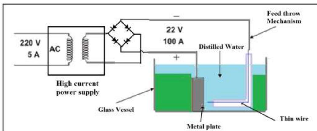
**Figure (1):** A schematic diagram of the electro-exploding wire (EEW)
