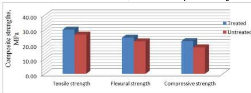
**Figure 1:** Effect of alkali treatment on the tensile, flexural and compressive strengths of the composites
