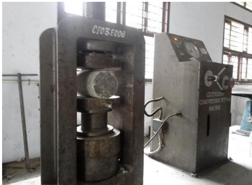
Figure 1: Split Tensile Strength Test Setup
