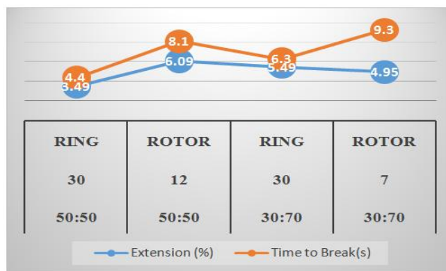
Figure 4. Yarn Extension and Time to Break of Different Blend Ratio (cotton-banana)
