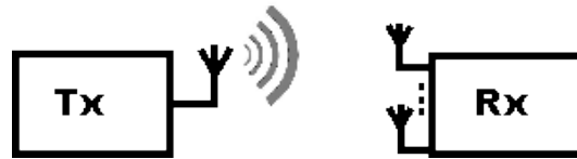
Figure 2 SIMO - Single Input Multiple Outputs
