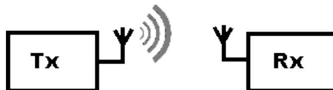
Figure-1 SISO - Single Input Single Output
