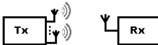
Figure -3 MISO- Multiple Input Single Outputs
