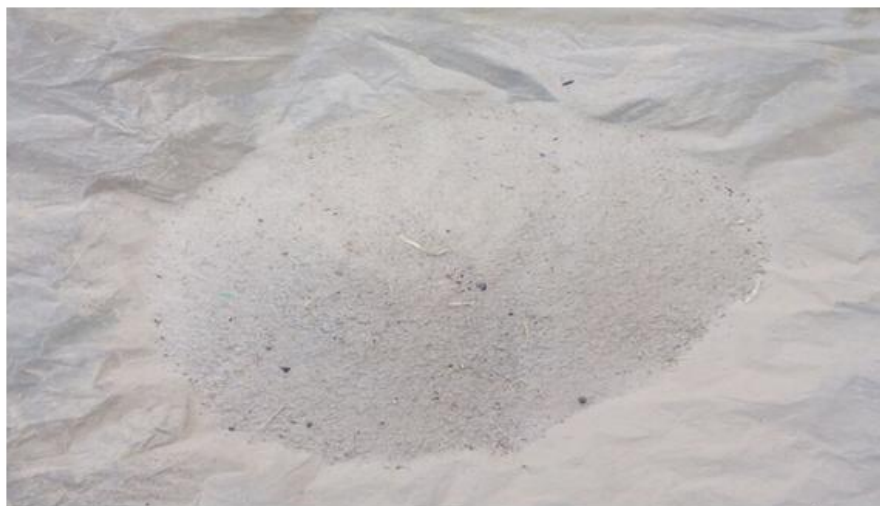
Plate 2 Waste glass in ground fine form after processing
