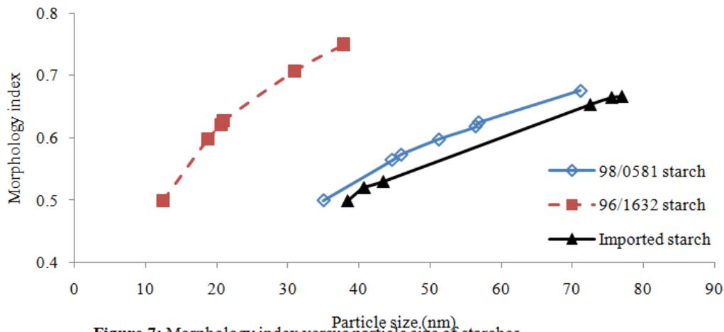
Figure 7: Morphology index versus particle size of starches
