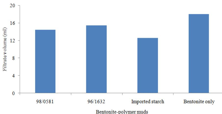
Figure 10: API fluid losses of bentonit-polymer muds
