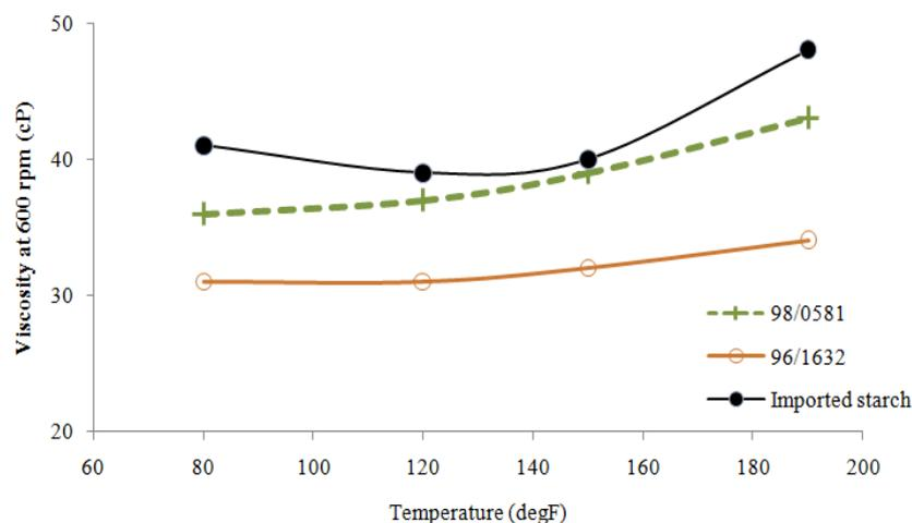
Figure 9: Viscosity bentonite-polymer mud at 600 rpm
