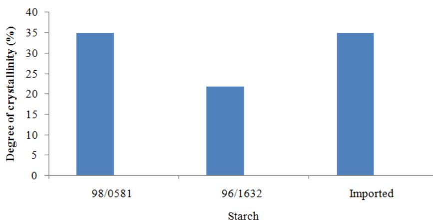
Figure 6: Degree of crystallinity of starches
