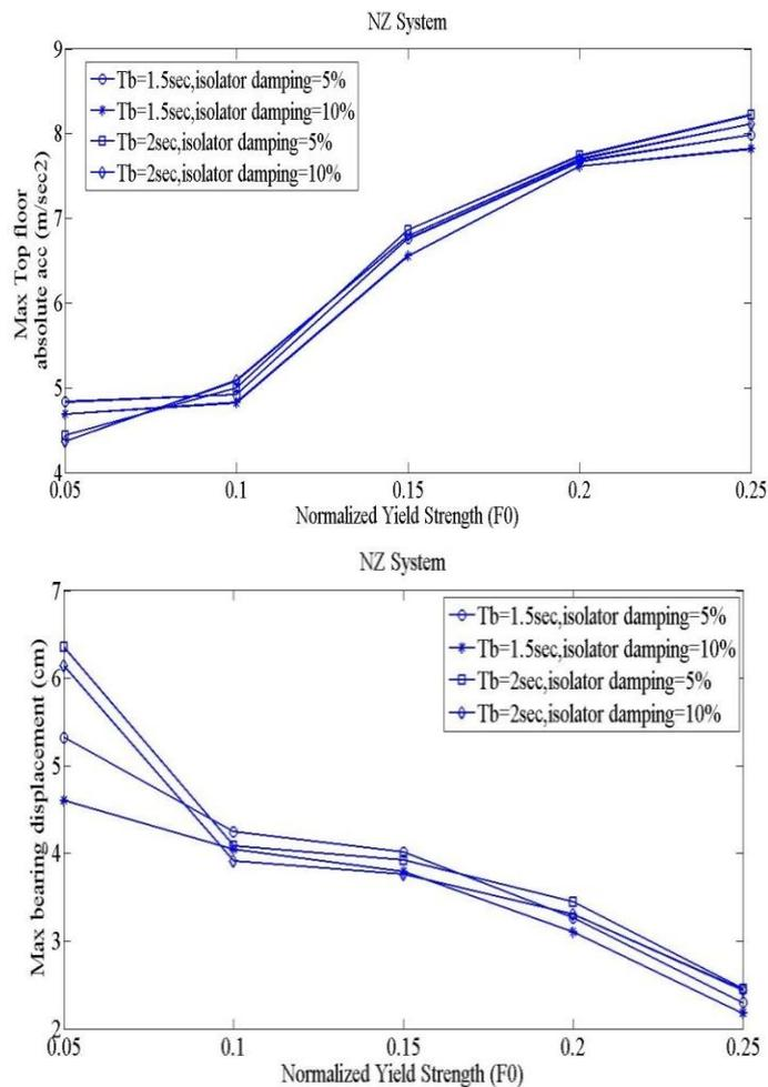
**Figure 9:** Effect of Normalized Yield Strength on top floor absolute acceleration and max. bearing displacement for building isolated by NZ bearing, Subjected to El Centro (1940) Earthquake
