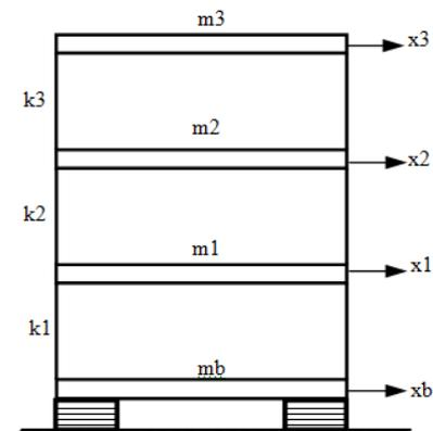
Figure 3: Model of Base Isolated building.
