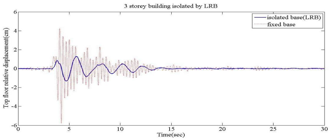
**Figure 6:** top floor relative displacement for fixed base building and for base isolated building isolated by laminated Rubber bearing ( $T_b$  2 sec,  $\zeta_b$  10%), Subjected to (a) El Centro (1940) Earthquake, (b) Kobe (1995) Earthquake, (c) Sylmar(1971) Earthquake
