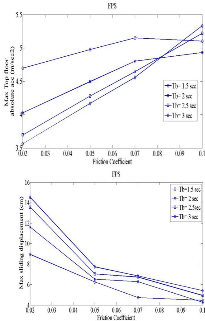
**Figure 10:** Effect of isolation time period( $T_b$ ) and Friction Coefficient ( $\mu$ ) on top floor absolute acceleration and max. bearing displacement for building isolated by FPS, Subjected to El Centro (1940) Earthquake
