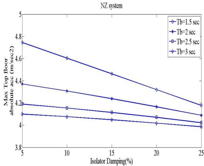
**Figure 8:** Effect of isolation time period and bearing damping ratio on top floor absolute acceleration and max. bearing displacement for building isolated by NZ bearing ( $F_0=0.05$ ), Subjected to El Centro (1940) Earthquake
