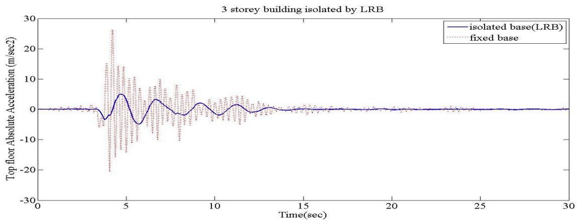
**Figure 5:** top floor absolute acceleration for fixed base building and for base isolated building isolated by laminated Rubber bearing( $T_b$  2 sec,  $\zeta_b$  10%), Subjected to (a) El Centro (1940) Earthquake, (b) Kobe (1995) Earthquake, (c) Sylmar(1971) Earthquake
