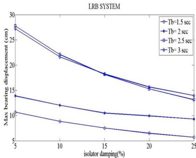
**Figure 7:** Effect of isolation time period and bearing damping ratio on top floor absolute acceleration and max. bearing displacement for building isolated by LRB, Subjected to El Centro (1940) Earthquake
