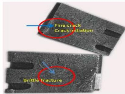
Fig. 5: Two broken pieces of die
