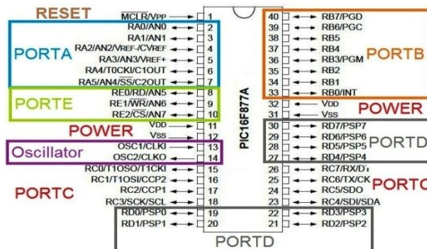
Figure 2: Pin configuration of PIC 16F877A
