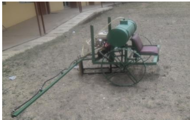
Plate 1: Assembled Prototype Sprayer
