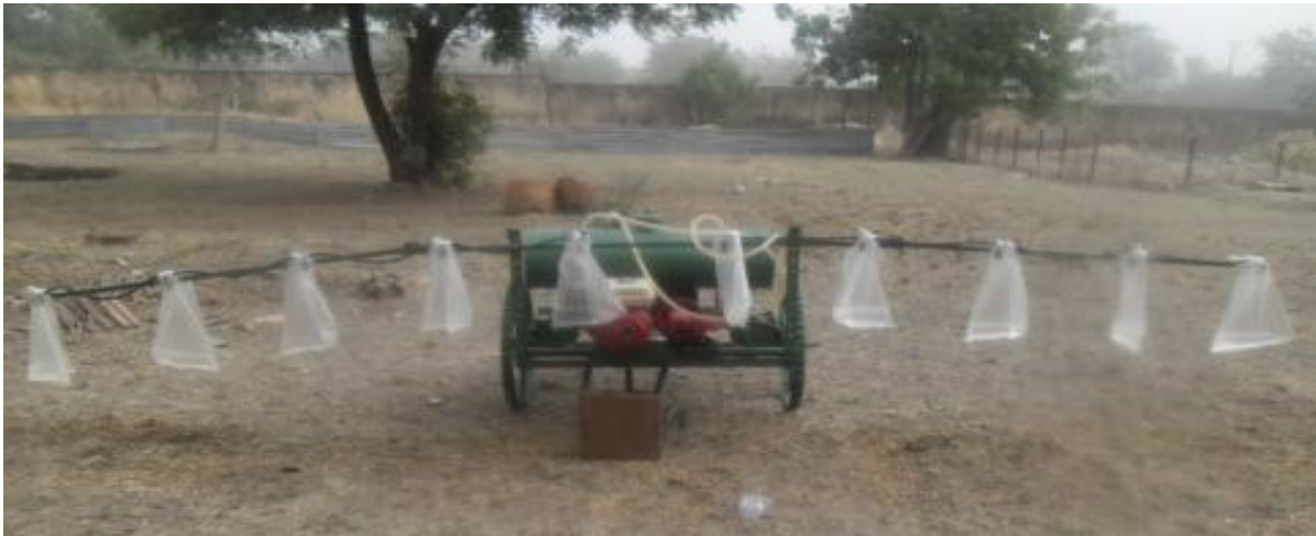
Plate 3: Measurement of Nozzle Flow Rate
