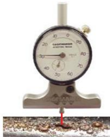
Fig. 7 The pit depth gage.
