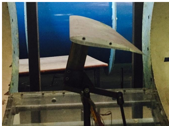
Figure 9, airfoil section in wind tunnel.
