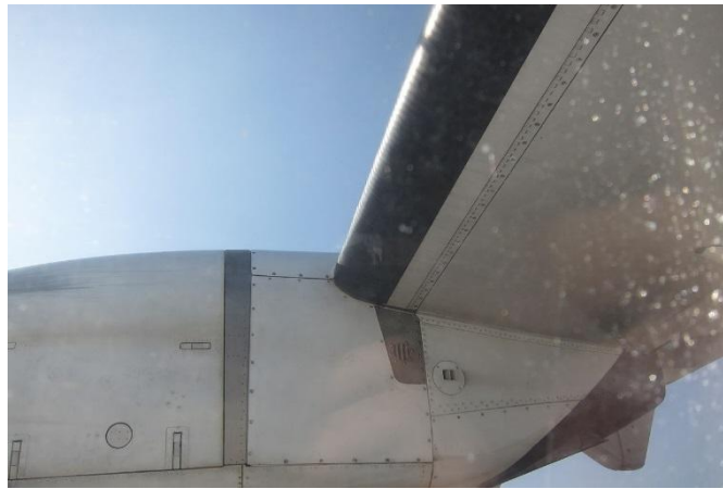
Figure 4, rubber leading edge for ice removal.
