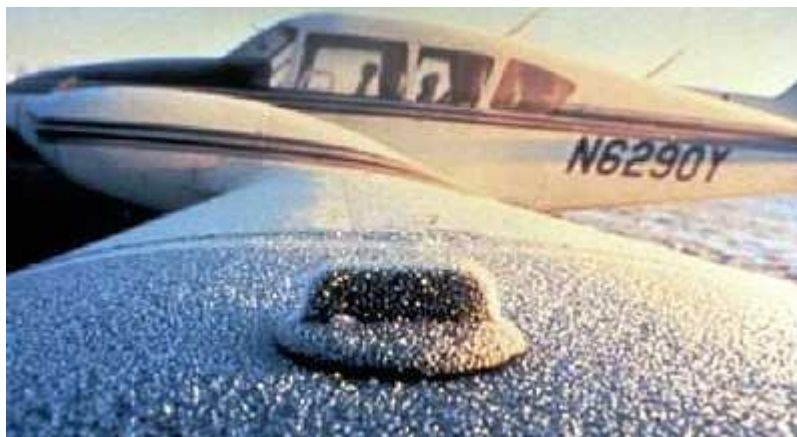
Figure 5, upper surface ice in flight.
