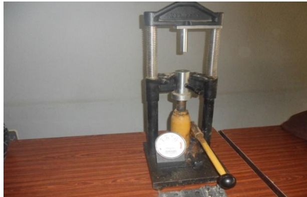
Figure 1: Manual hydraulic press fixed with a pressure gauge
