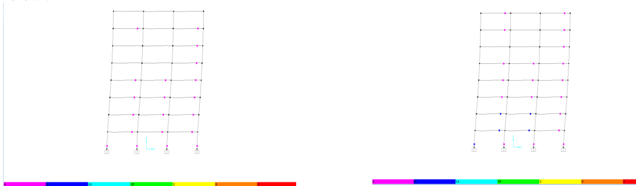
Fig. 10. display plastic joints of frame S28 Modeling in SAP software and under the pushover analysis with displacement of goal obtained from scaled method with range 2800 standard plan and with spectral acceleration of curve 50% obtained from IDA analysis corresponding to the maximum relative displacement between floors 1%
