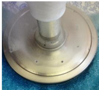
Fig. 15. Photo of moisture extraction process from the porous material
