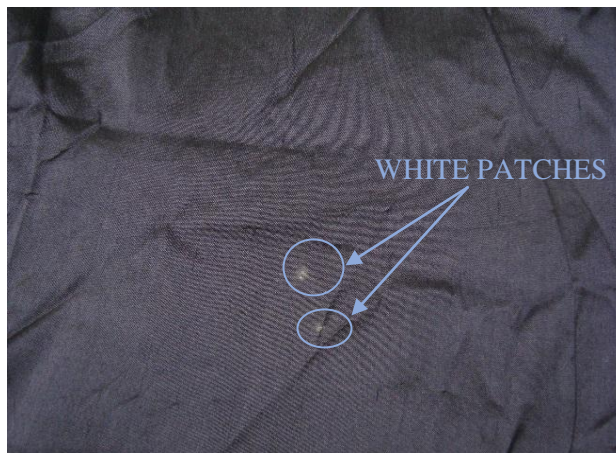
Fig.1 occurrence of white patches on the surface of the dyed silk fabric
