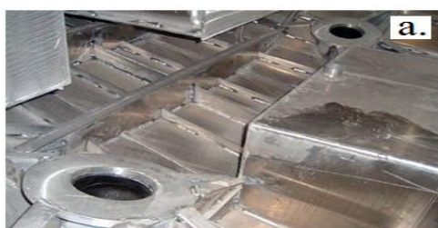
Figure 1 a. The bearing welded into a tube in an aluminium hull, [5] and b. the properties of aluminium versus steel[6].
