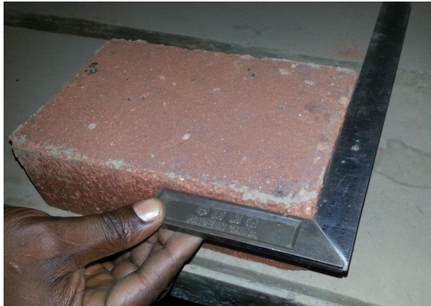
Figure 3.2 Dry Block being checked with Try Square
