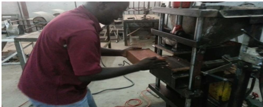
Figure 2.5 Compressed Soil Block lifted to curing yard
