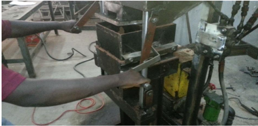
Figure 2.4 Soil Mix being fed into Mould from hopper
