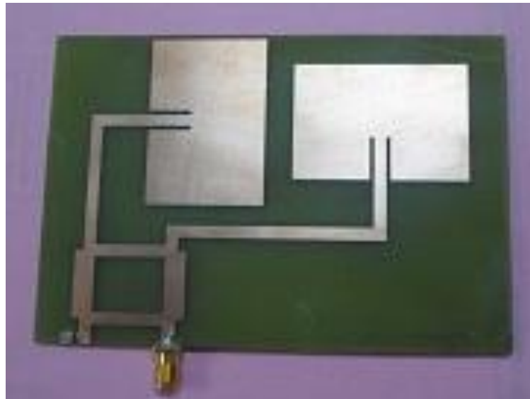
Figure 7. Photograph of fabricated antenna
