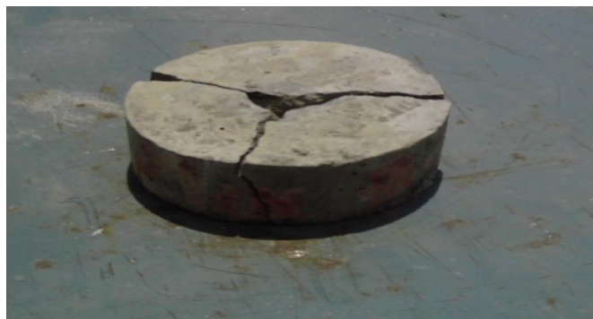
Figure 2: Plain Concrete Specimen
