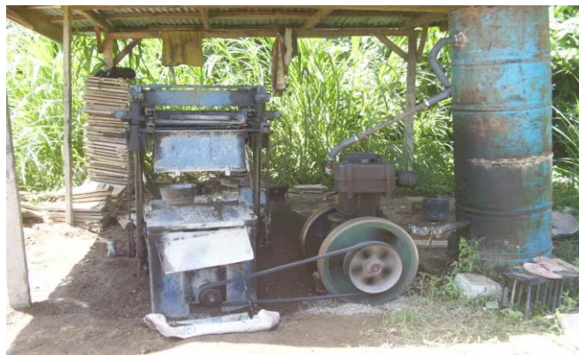
Figure 3: A diesel powered engine machine-compacted mould
