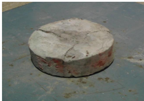
Figure 3: Polypropylene fibre Concrete Specimen
