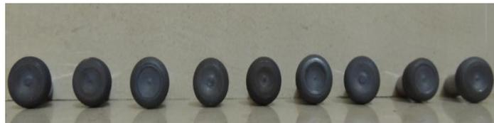
**Fig 4.5 Diameter of mechatrode after friction surfacing**
