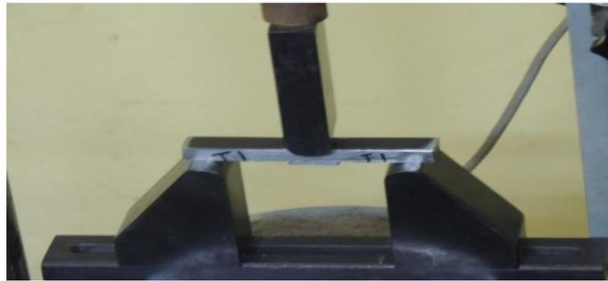
Fig 5.4 Sample before the bend test
