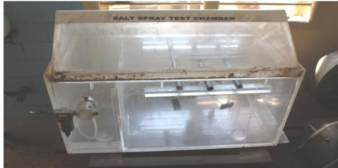
Fig 5.6 Salt spray test chamber apparatus
