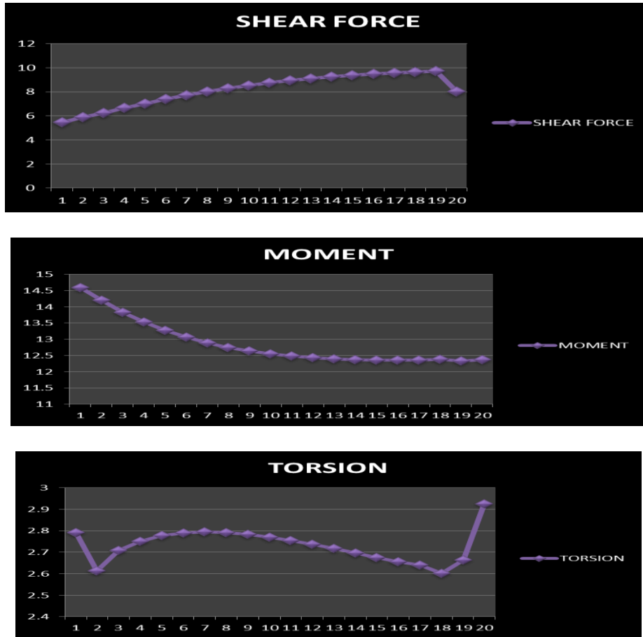
Figure 8: Shear Force, Torsion and Moment for Beam B20
