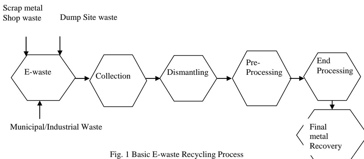
Fig. 1 Basic E-waste Recycling Process
