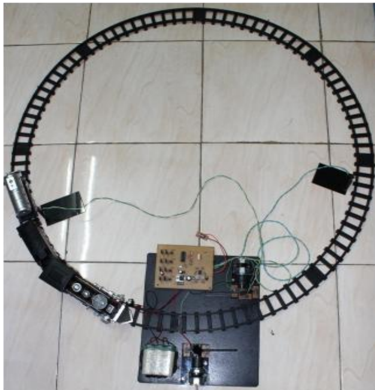
Fig. 15. An automatic railway gate control
