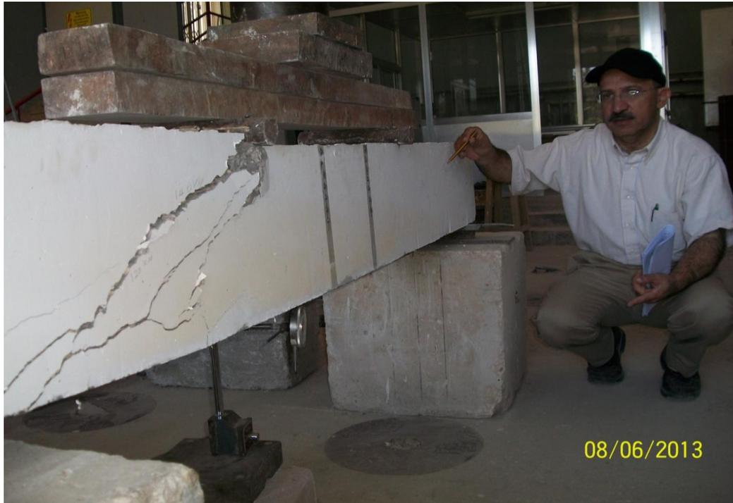
Figure 6: Beam BU at failure stage
