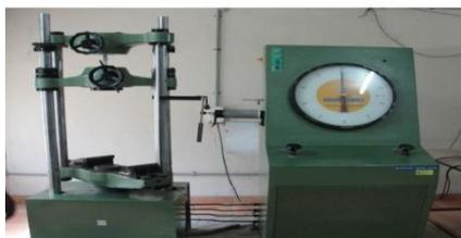
Fig 2: Universal Testing machine
