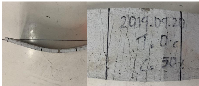
ECC-RBP2: Recycled brick powder 50%, Quartz sand 50%, Temperature 0°C
