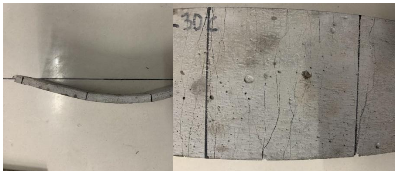
ECC-RBP2: Recycled brick powder 50%, Quartz sand 50%, Temperature -30°C
