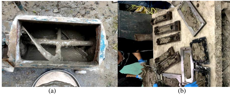
Fig. 4. Shaft mixer and vibration table: (a). shaft mixer, (b). vibration table
