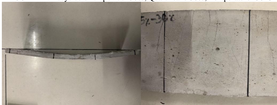
ECC-RBP3: Recycled brick powder 75%, Quartz sand 25%, Temperature -30°C
