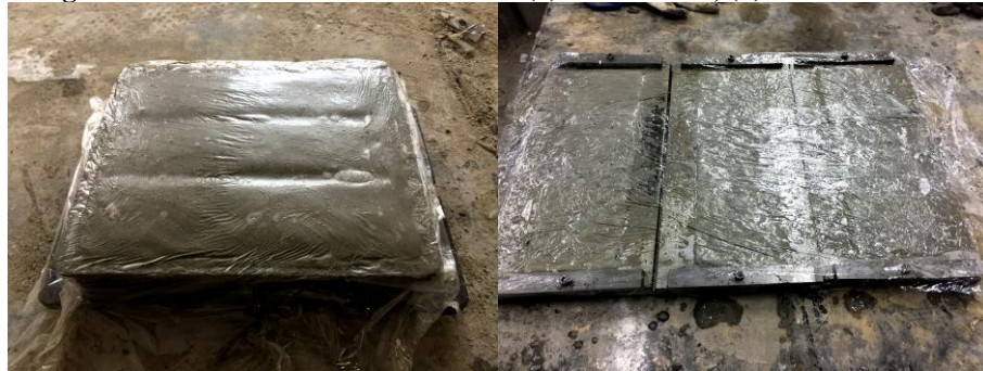
Fig. 5. Photo of covered with plastic film
