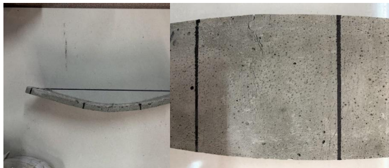
ECC-NC: Recycled brick powder 0%, Quartz sand 100%, Temperature -10°C
