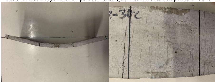
ECC-RBP1: Recycled brick powder 100%, Quartz sand 0%, Temperature -30°C
