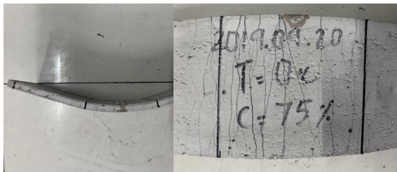
ECC-RBP3: Recycled brick powder 75%, Quartz sand 25%, Temperature 0°C
