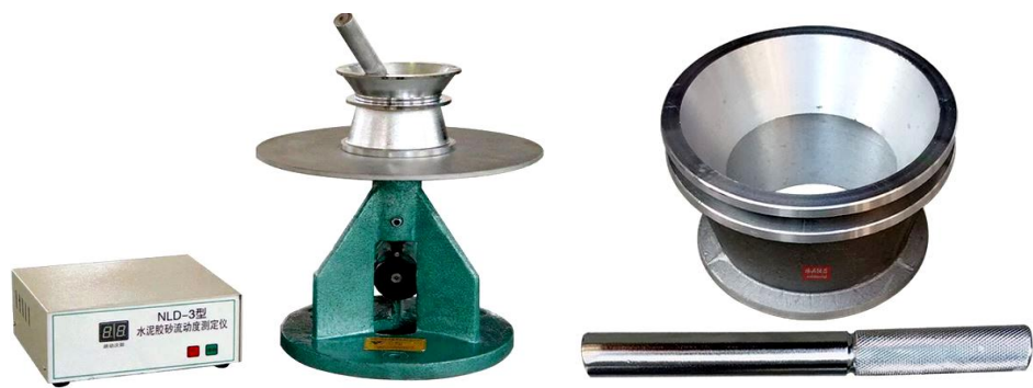
Fig. 8. Cement mortar fluidity tester
