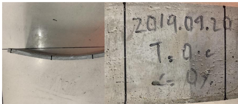
ECC-NC: Recycled brick powder 0%, Quartz sand 100%, Temperature 0°C
