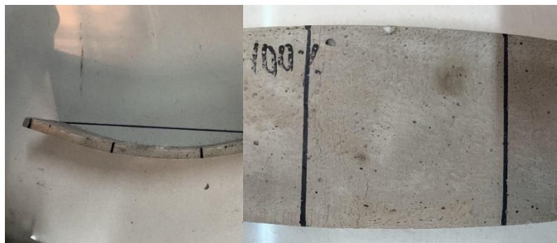
ECC-RBP3: Recycled brick powder 100%, Quartz sand 0%, Temperature -10°C
