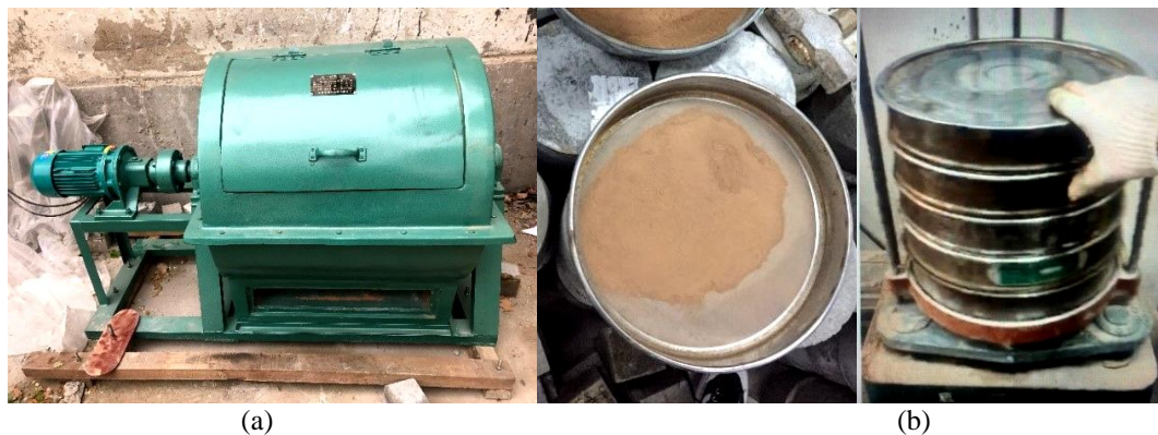
Fig. 3. Crushing and screening machine: (a). Crushing machine; (b). Screening machine
