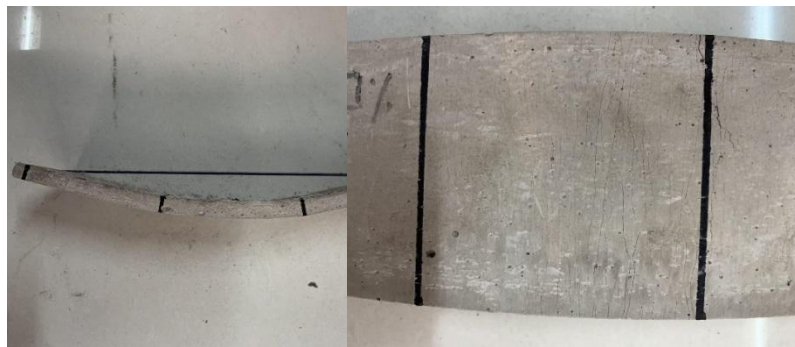
ECC-RBP4: Recycled brick powder 100%, Quartz sand 0%, Temperature -20°C
