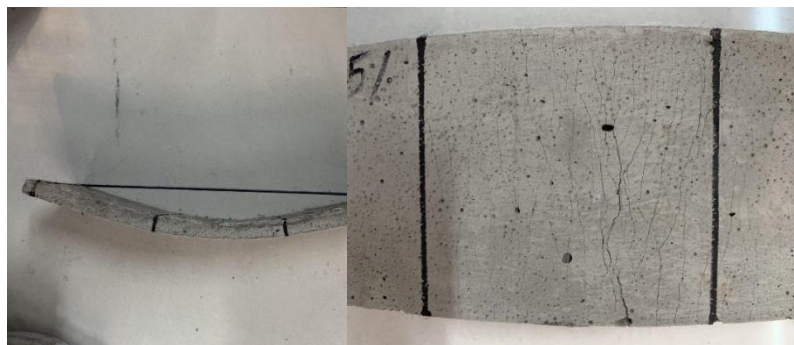
ECC-RBP1: Recycled brick powder 25%, Quartz sand 75%, Temperature -10°C
