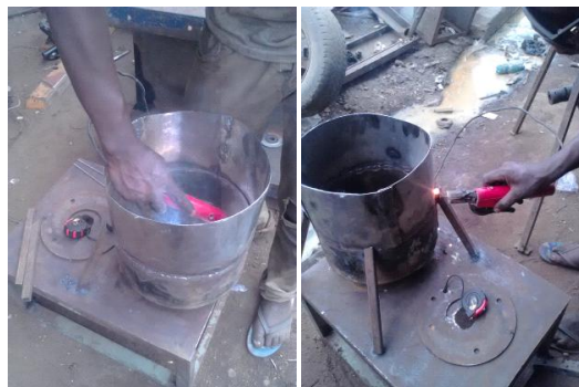
Plate 3 Welding the Supports of the Lacerating chamber
