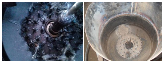
Plate 4 Spike unit in the lacerating chamber
