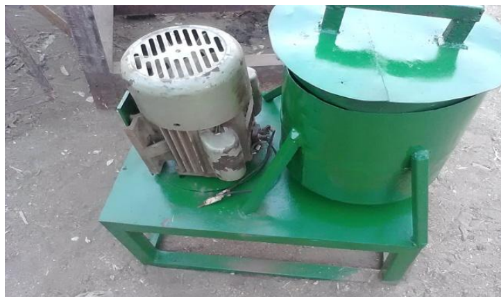
Plate 6 The fabricated water sachet lacerating machine
