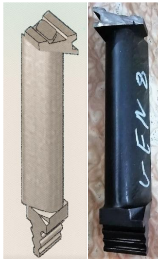
Figure. 1. shows the actual blade and computerized modeling aided by Inventor, modeling illustrates all designed dimensions of blade [8] [2].
