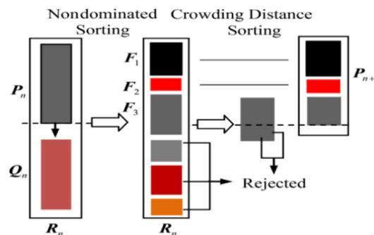
Figure 3. NSGA-II procedure
