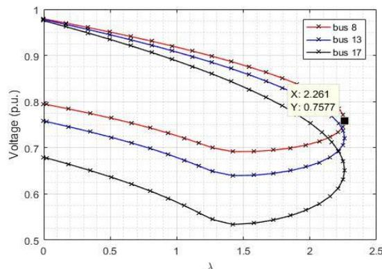
**Figure 9. PV-curve with D-STATCOM**
