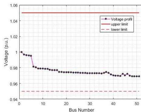
Figure 7. Voltage profile with D-STATCOM at bus 37
