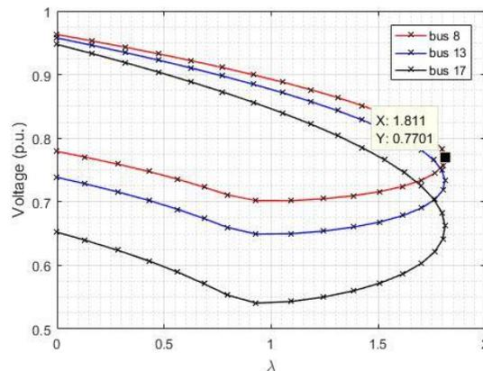
**Figure 8. PV-curve without D-STATCOM**
