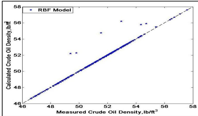
Fig. 2. Accuracy of RBF crude oil density model for testing
