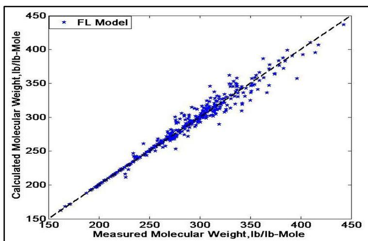
Fig. 12. Accuracy of FL molecular weight model for testing
