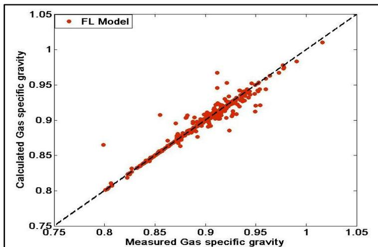
Fig. 7. Accuracy of FL gas specific gravity model for training
