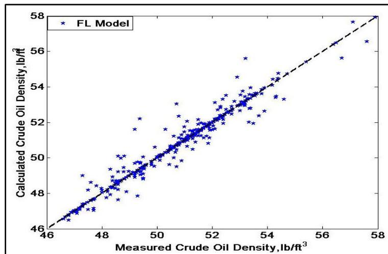
Fig. 4. Accuracy of FL crude oil density model for testing
