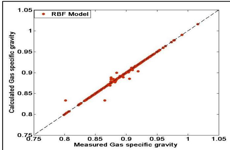
Fig. 5. Accuracy of RBF gas specific gravity model for training
