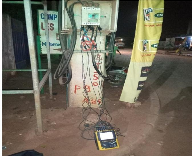
**Figure 2:** View of analyzer installation for measurements.
