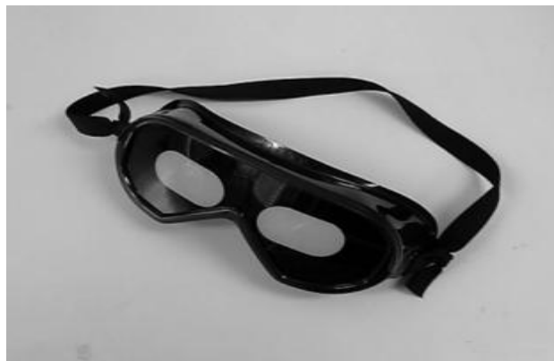
Fig. 2. Experimental equipment (Cataract reproduction goggles)
