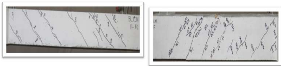
Fig.6. Side view of beam B1N at failure Fig.7. Side view of beam D1N at failure
