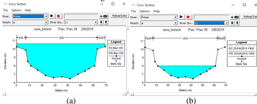
**Figure 16** Upstream conditions of the primary canal at (a) high tide and (b) low tide
