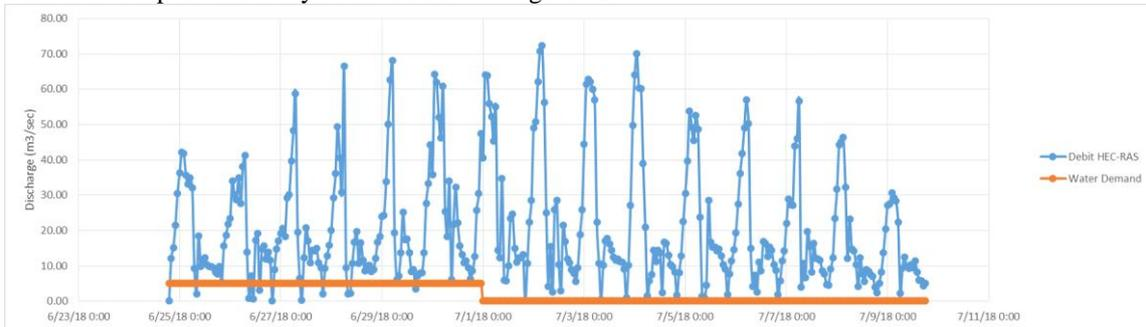
Figure 28 DIR Belanti I water balance (HEC-RAS discharge vs. water demand)
