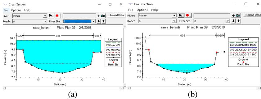
Figure 17 Condition of the primary channel downstream during (a) high tide and (b) low tide
