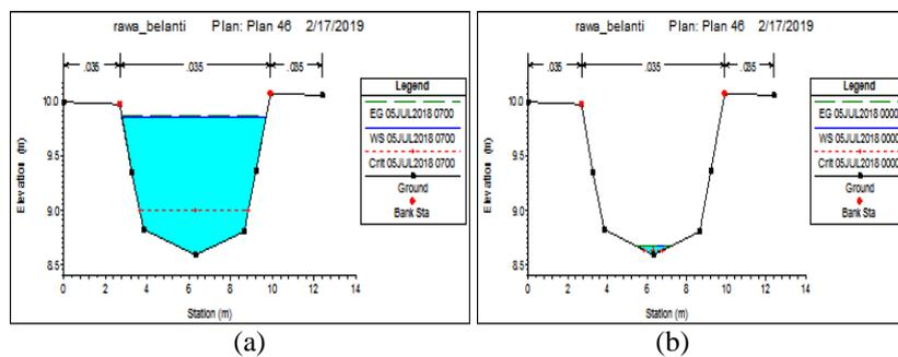
Figure 22 Condition of downstream secondary channel 1 at (a) high tide and (b) low tide
