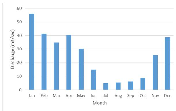
Figure 13 80% Reliable discharge
