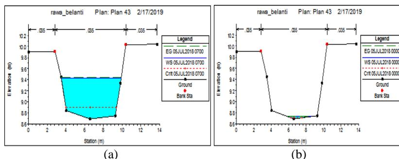
Figure 23 Condition of the downstream secondary canal at (a) high tide and (b) low tide
