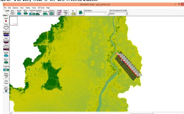
**Figure 8** Geometry DIR I BELANTI on the HEC-RAS
