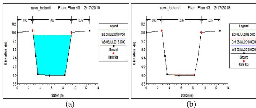
Figure 21 Upstream conditions of the right secondary channel at (a) high tide and (b) low tide
