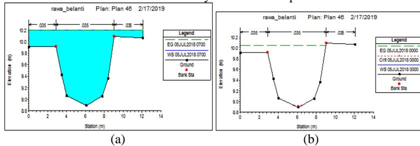
Figure 20 Upstream conditions of the left secondary channel 1 at (a) high tide and (b) low tide
