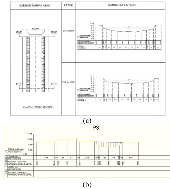
Figure 7 Cross-section (a) primary channel; (b) secondary channels
