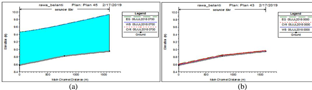
Figure 25 Long-section sek. 50 left (a) high tide; (b) low tide
