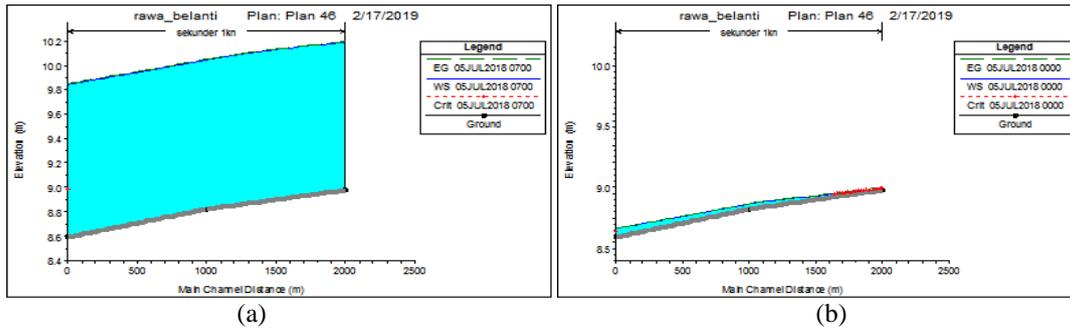
Figure 24 Long-section 1 right (a) high tide; (b) low tide
