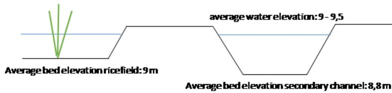
Figure 27 Sketch of ricefield elevation and secondary channel elevation.
