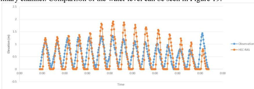
Figure 19 Tidal graph downstream of the primary channel (HEC-RAS vs. Observation)
