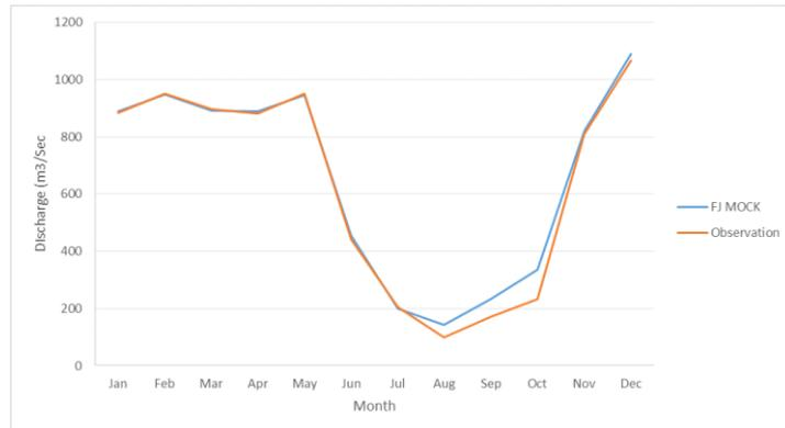
Figure 12 Comparison of FJ Mock discharge and measured discharge
