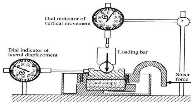
Fig 1: Schematic illustration of the shear box testing apparatus (Source: Slide 21 Geotechnical Engineering and Soil Mechanics Laboratory Manual, Texas Tech University)
