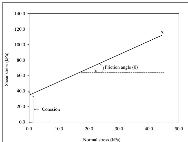
Fig 3: Shear stress and normal stress relation with correlation coefficient of 0.986
