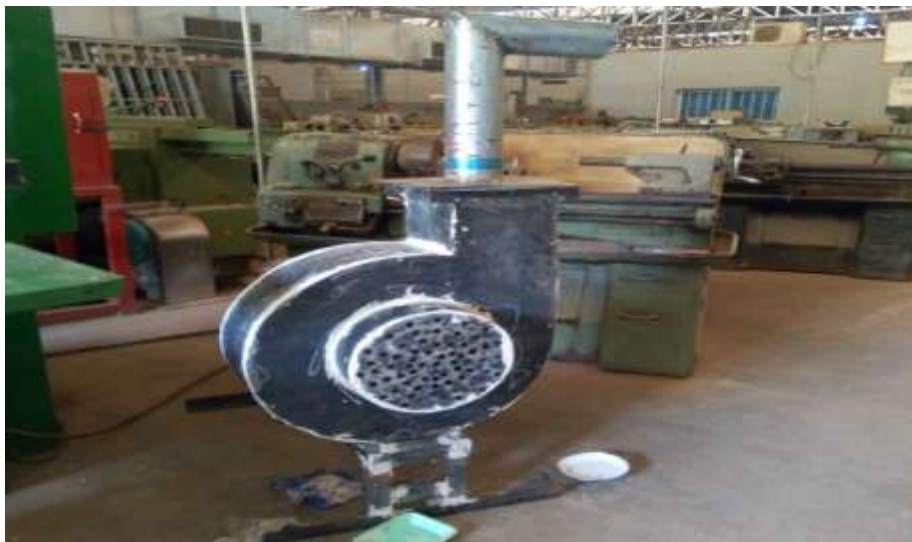
FIG 2 Assembled blower with housing
