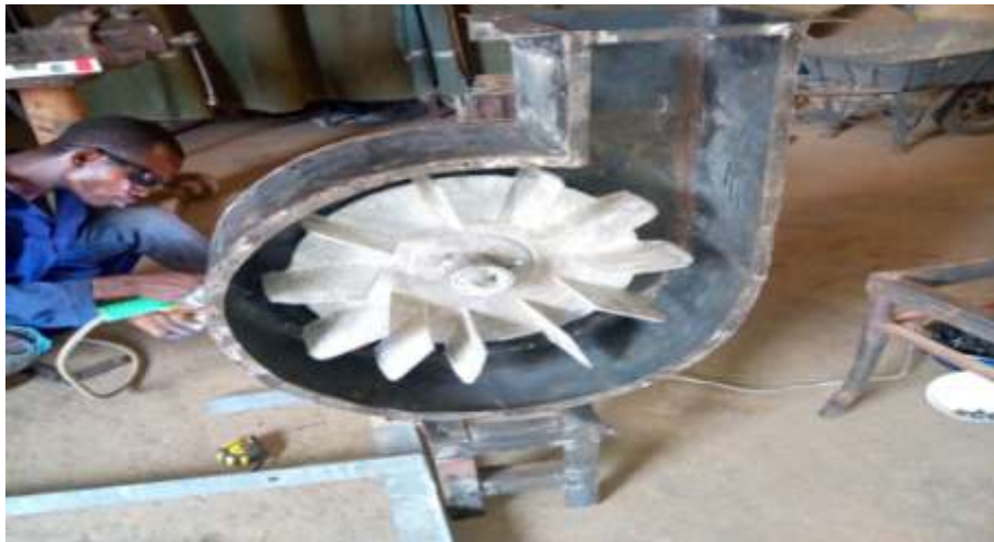
FIG1 Casing showing the casted aluminium scrap blades
