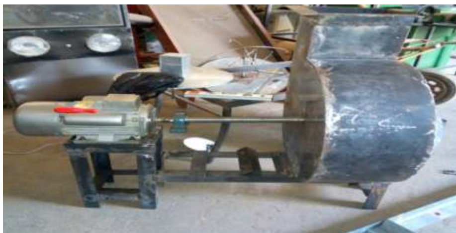
Fig 3 Assembled blower with housing and electric motor
