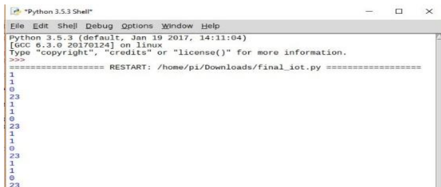
Fig. 5. Received sensor data in Raspberry Pi (View on Python shell 3.5.3)
