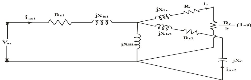
Figure 2. Steady State Equivalent Circuit.
