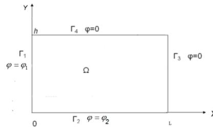
FIG. 1 – Rectangular plate and boundary conditions
