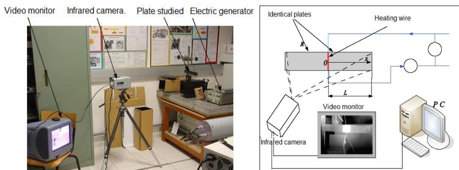
**FIG. 2** – Fitting the experimental measurement of the temperature.
