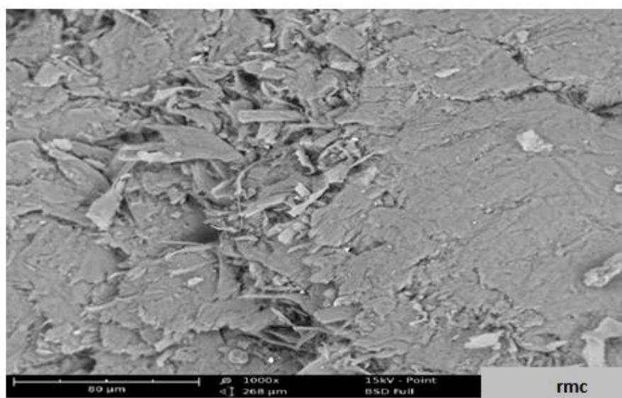
**Fig. 2a:** SEM image of raw maize cob at 1000x
