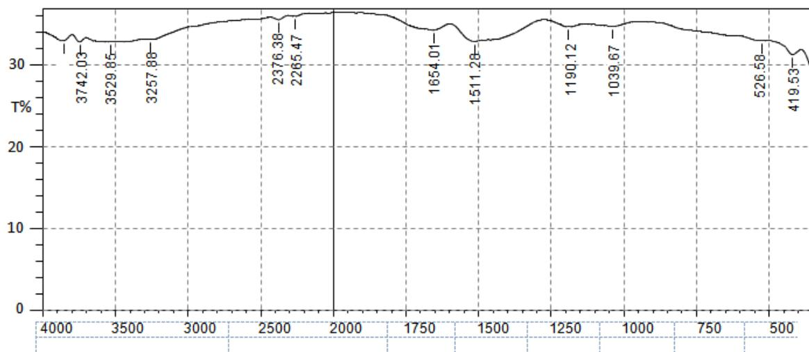
**Fig. 1:** FTIR spectra of rmc powder
