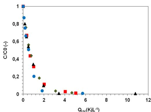
**Figure 9:** Evolution of the pyrimethanil concentration as a function of the accumulated energy per liter of solution to be treated with the catalyst P-25
