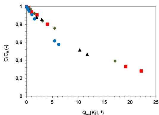
**Figure 10:** Evolution of the pyrimethanil concentration as a function of the accumulated energy per liter of solution to be treated with the catalyst Ahlstrom
