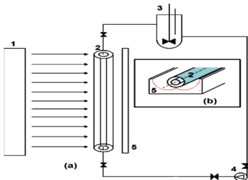
Figure 1: Diagram of the driver used. (5), Pump (4), UV lamp (1), Reactor (2), Storage tank
