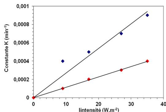
**Figure 8:** Evolution of the degradation kinetics of pyrimethanil (◆) and TOC (◆) as a function of the irradiation ( $WUV.m^{-2}$ ) by the catalyst Ahlstrom
