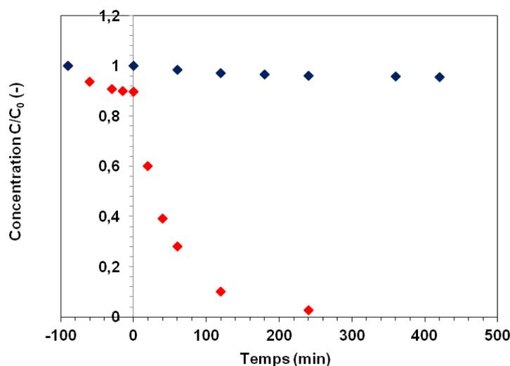
**Figure 2:** Kinetics of the disappearance of pyrimethanil in the absence of the catalyst (♦) (photolysis); Adsorption of pyrimethanil ( $t < 0$ ); Photocatalytic treatment in the presence of TiO<sub>2</sub> / UV (♦) for  $t > 0$ . Influence of irradiation on the Degussa P-25
