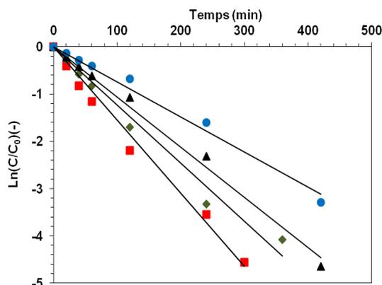
**Figure 5:** Expression of the logarithm of the relative pyrimethanil concentration as a function of time (min) for different irradiations ( $WUV.m^{-2}$ ): 9(●), 17(▲), 27(◆),35(■) by the catalyst P-25
