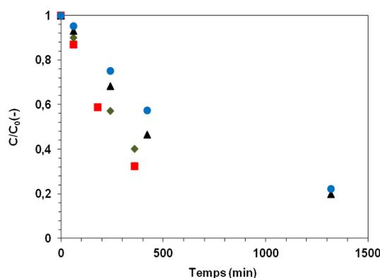
Figure 4: Evolution of the relative TOC concentration as a function of time (min) for different irradiations (WUV.m-2): 9(●), 17(▲), 27(◆), 35(■)
