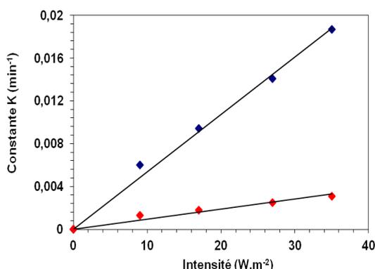
**Figure 7:** Evolution of the degradation kinetics of pyrimethanil (◆) and TOC (◆) as a function of the irradiation ( $WUV.m^{-2}$ ) by the catalyst P-25
