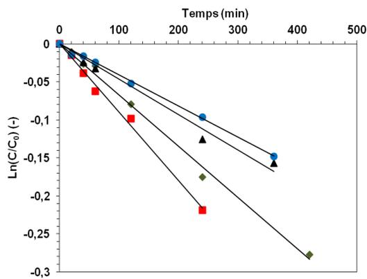
**Figure 6:** Expression of the logarithm of the relative pyrimethanil concentration as a function of time (min) for different irradiations ( $WUV.m^{-2}$ ): 9(●), 17(▲), 27(◆),35(■) by the catalyst Ahlstrom
