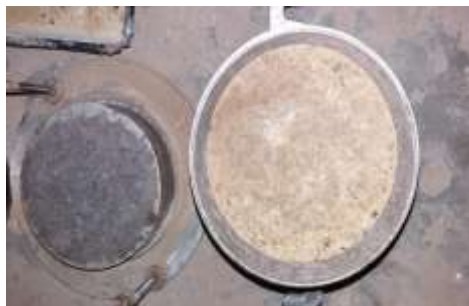
Figure 2: CBR Test Mix Composition in Mould
