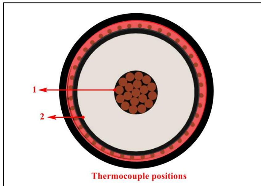
Fig. 4. The location for each thermocouple in the cable
