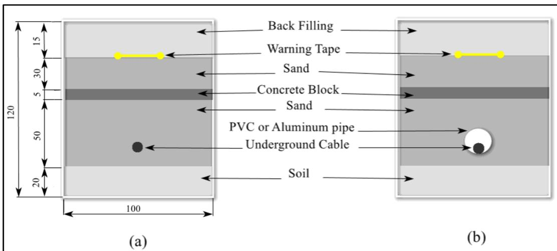
Fig. 2.Underground cable installations for the three models, all dimensions in cm
