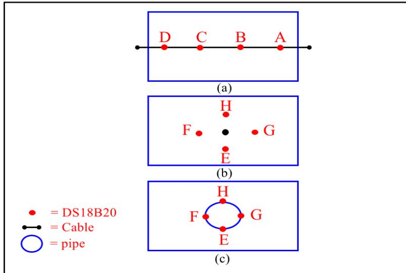
Fig. 5.The representation of the location for each sensor in (model 1, 2 and 3)
