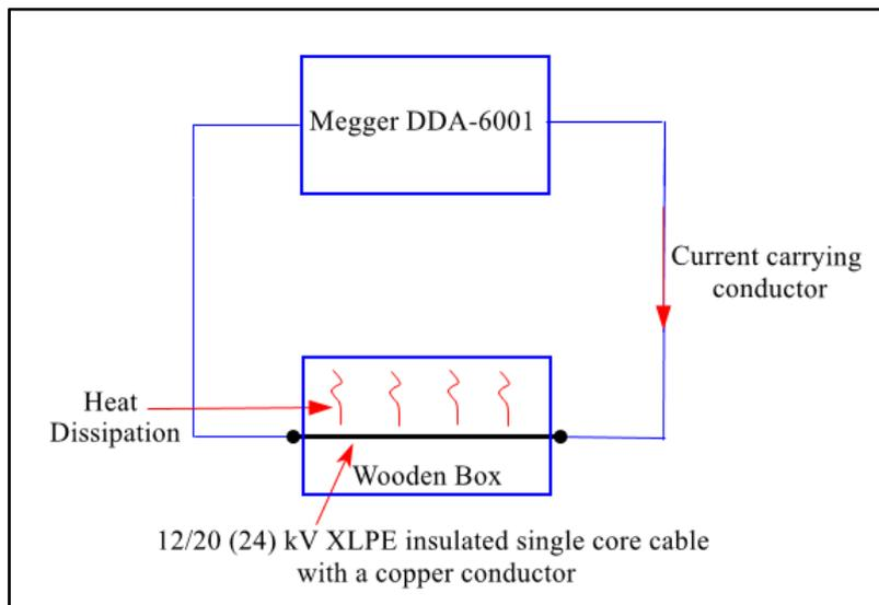
Fig. 6.Overview of the experimental structure
