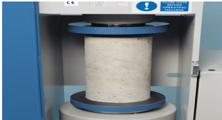
Fig. 3. Typical specimen cylinder inside the compression testing machine
