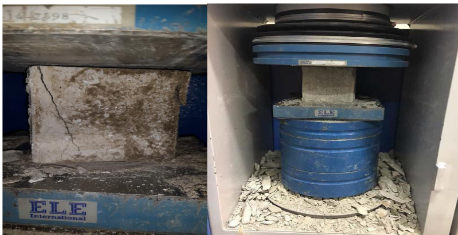
Fig. 2. Typical cube specimen failure mode under compressive testing of the cube
