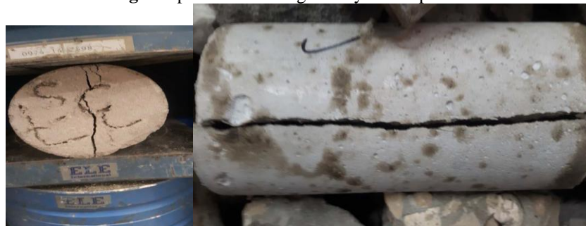
Fig. 7. Failure pattern of cylinder under splitting tensile strength (Indirect)
