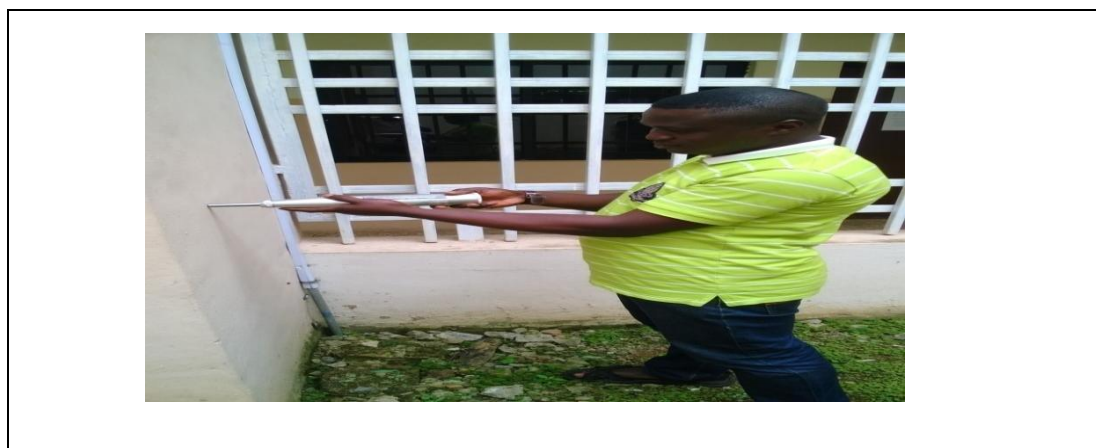
Plate 9: Picture showing the schmidthammer reading of ground floor column
