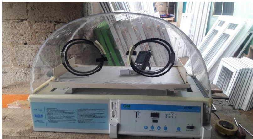
Figure 7: Experimental set up of baby incubator with hemispherical hood
