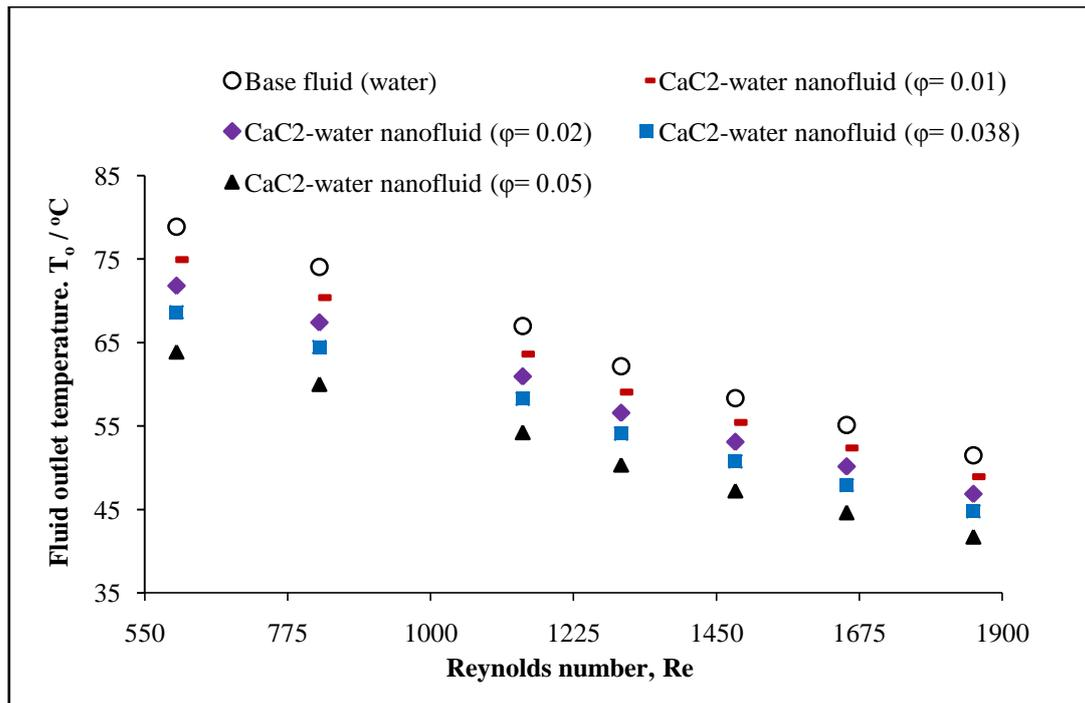
Fig. 5: Effect of nanoparticle volume fraction on fluid outlet temperature
