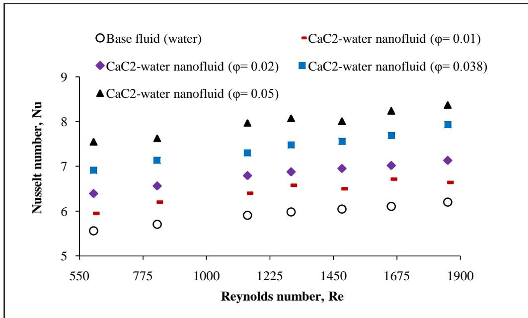
Fig. 3: Nusselt number at various nanoparticle volume fraction and Reynolds number
