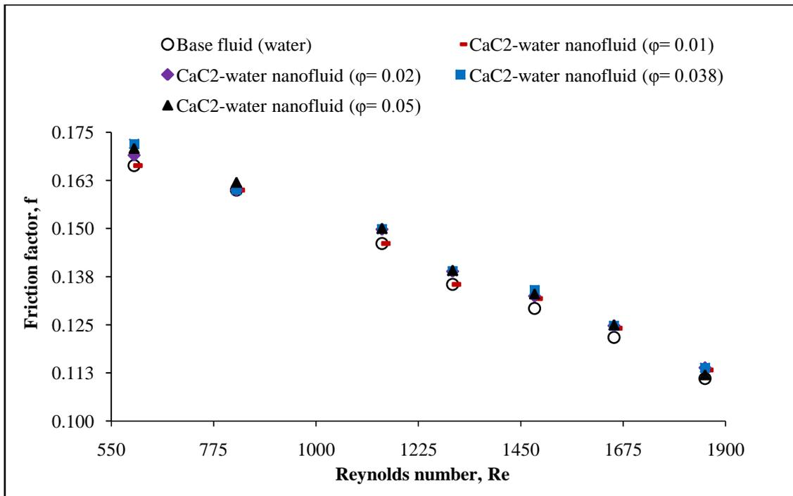
Fig. 4: Friction factor at various nanoparticle volume fraction and Reynolds number
