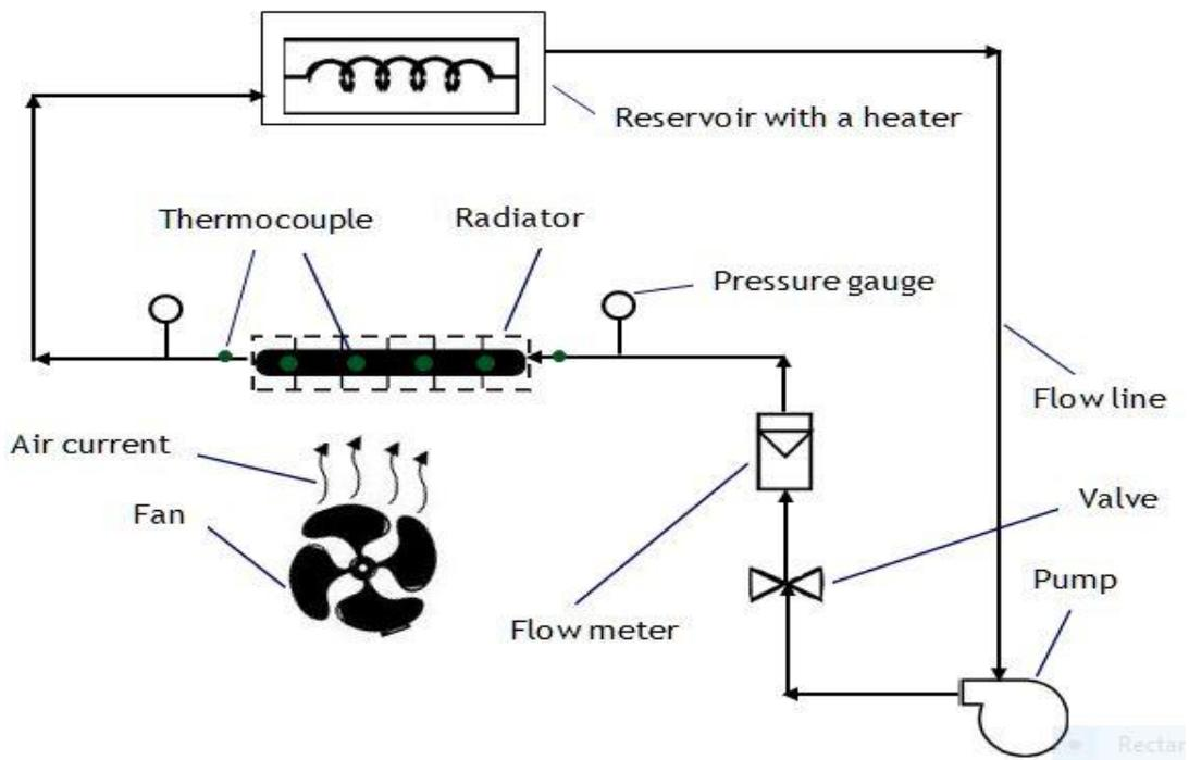
Fig. 1: Schematic diagram of components of the experimental system
