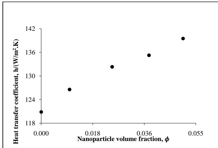
Fig. 2: Heat transfer coefficient at various nanoparticle volume fraction
