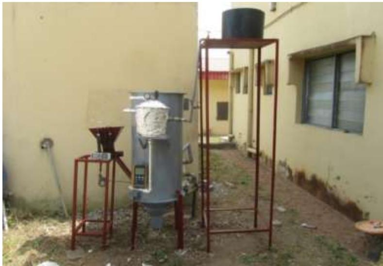
Figure 4. Fabricated PKS Combusting Furnace
