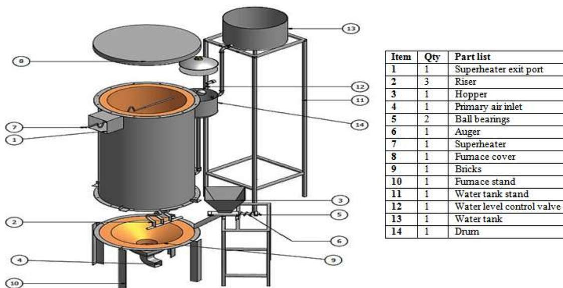
Figure 3. Exploded view of the developed PKS Combusting Furnace Unit
