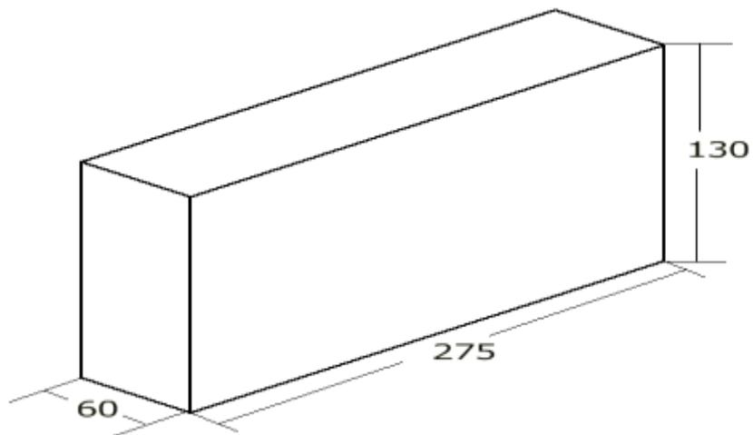
**Figure 2. Refractory brick**
