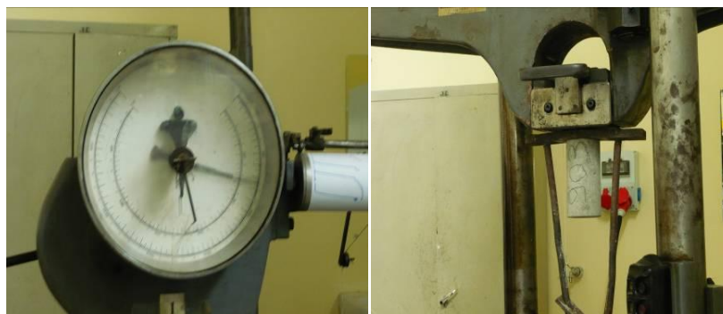
Fig. 2. Setup of the pullout testing system.
