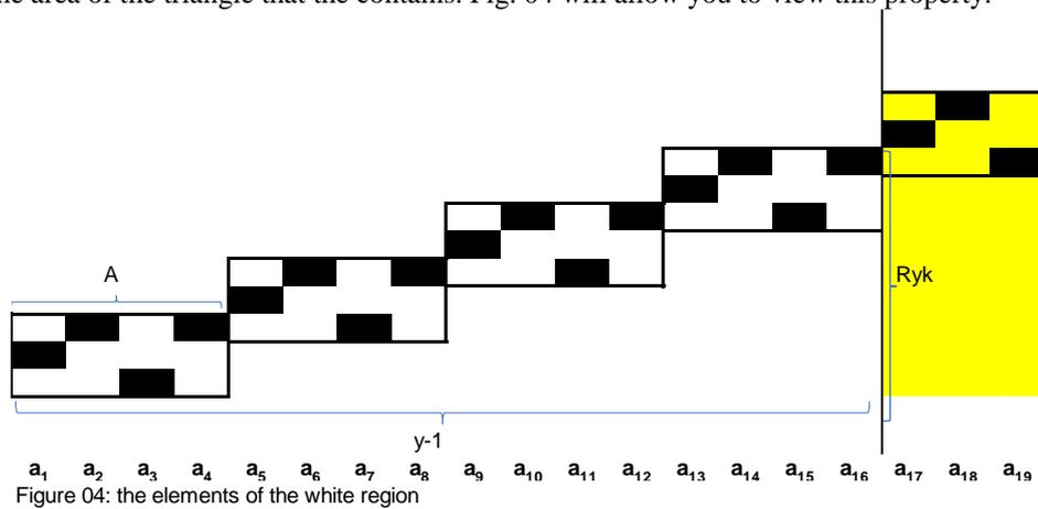
The base of the triangular region is given by  $y - 1$  times, its height is given by the product of step height  $R$ , by the cycle where they are  $y$ , and the quantity of ratios or values in each cycle  $k$ , thus being the area of the region white ( $Wa$ ) is expressed by:
